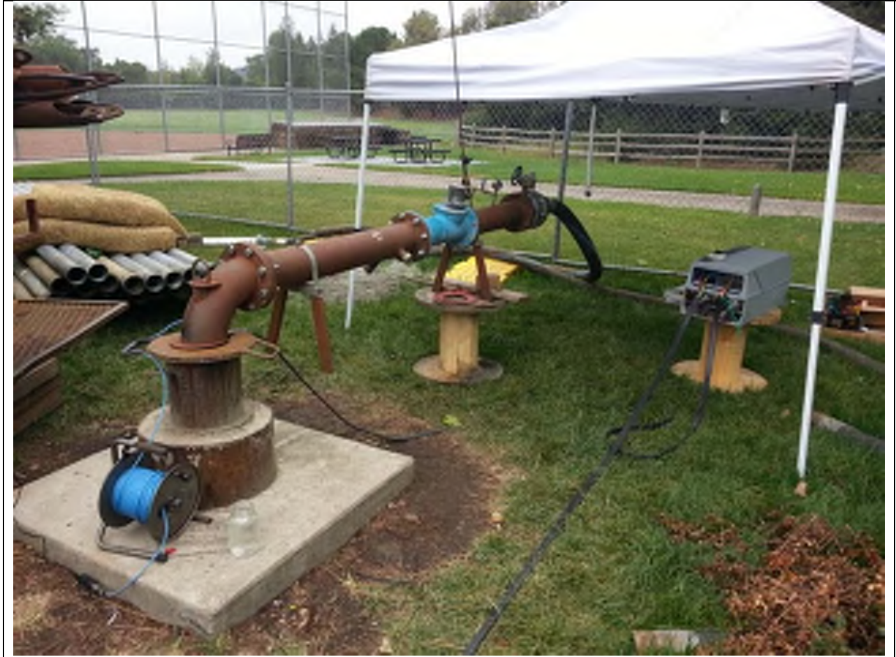
Configuration of well head during pumping tests.
