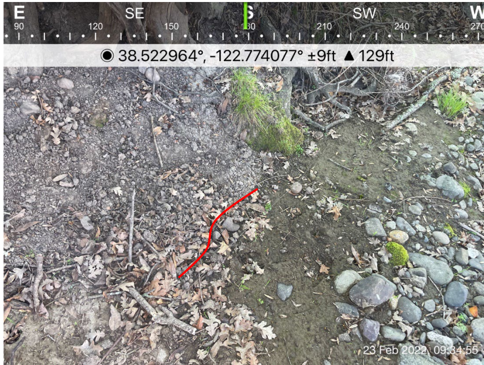
Photograph 13: Photo shows changes in soil character (red line), an indicator of OHWM, along Pruitt Creek.
