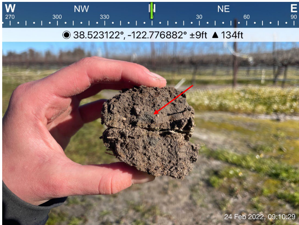
Photograph 8: Photo shows redoximorphic depletions (red arrow) within soils from wetland Sample Point 2B.
