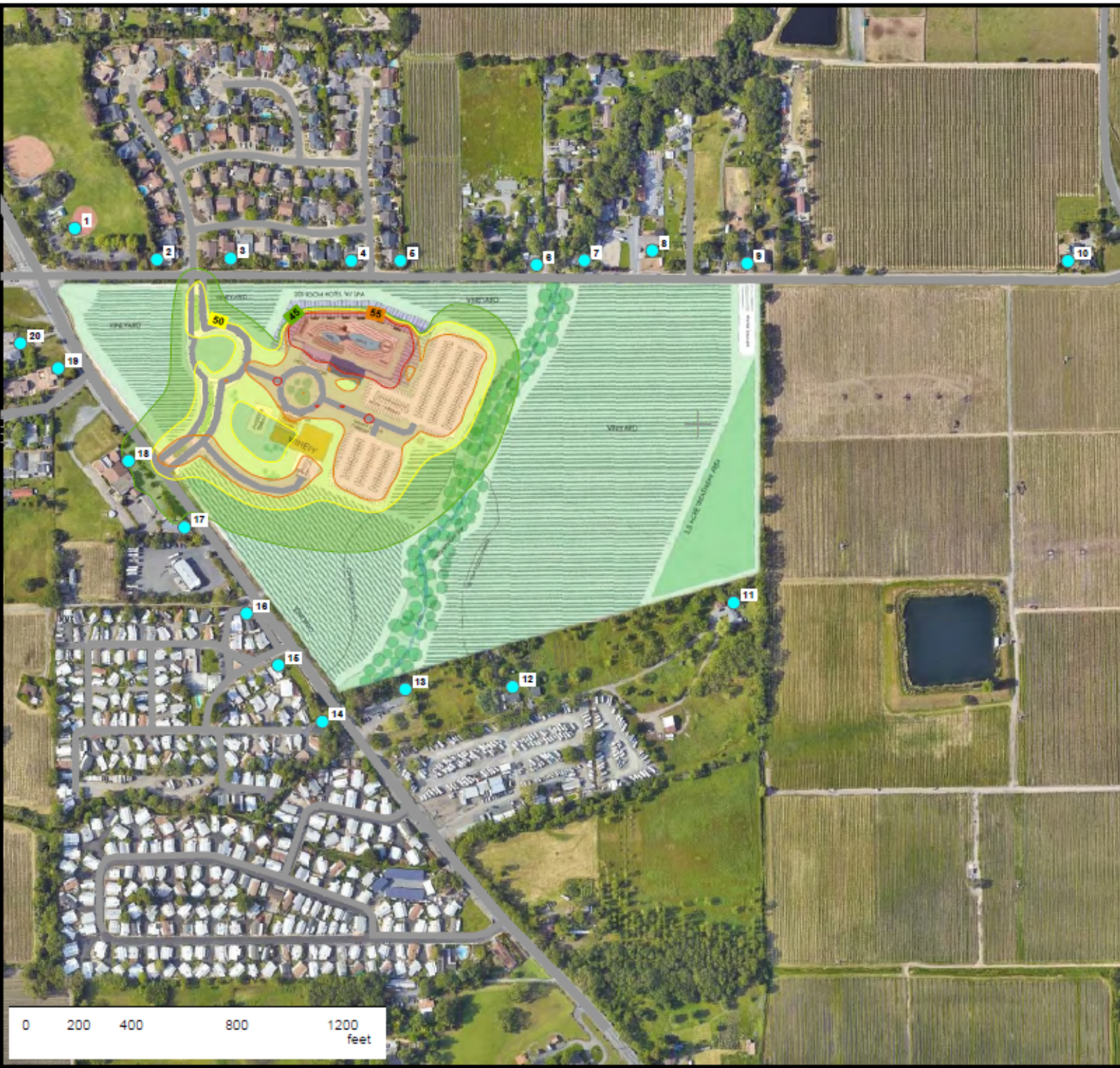
Figure 9 Shiloh Resort & Casino Alternative C Noise Contours ( L_{eq}/L_{50} ) for from combined noise sources: pool area, on-site traffic, passenger parking, and truck loading docks.
