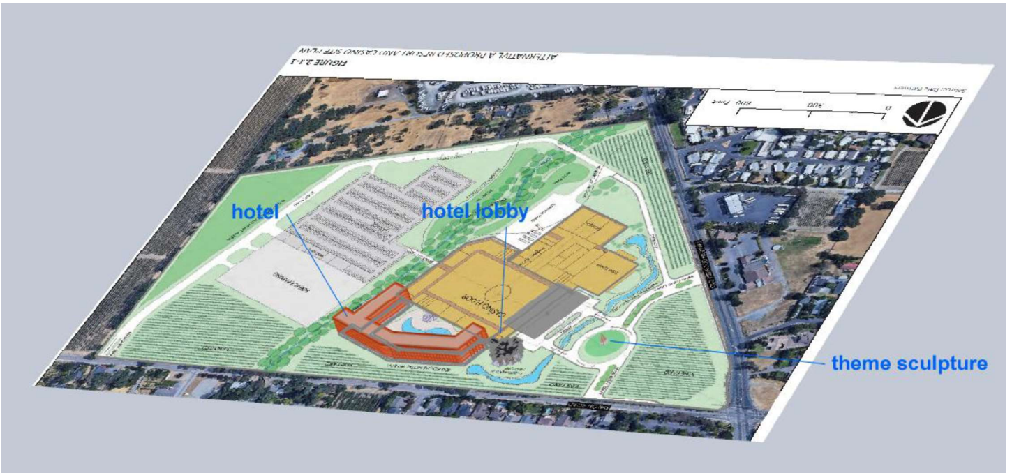
Figure 4. Development of a 3D CAD model of the project based on the site plan.
